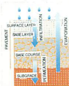
How water-permeable paving works
